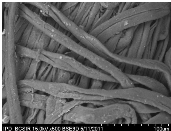
Fig 2(a). Scanning electron micrograph of denim garment after bleach treatment.
